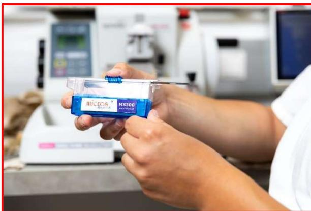
2. With extreme caution, insert the device into the microtome blade holder, still using the provided lever, in order to facilitate insertion. If the dispenser does not eject the blade, do not force it to come out.
